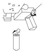
Remove the protective plug from the end of the new cartridge.
