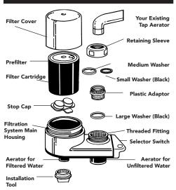
Use R2 replacement cartridge with F2 filter model.
